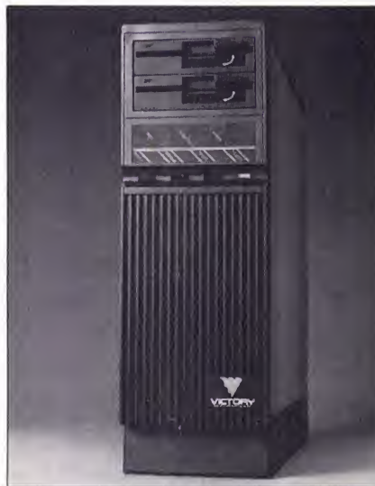
The Victory MicroFactor II is a 68000-based System V supermicro.
