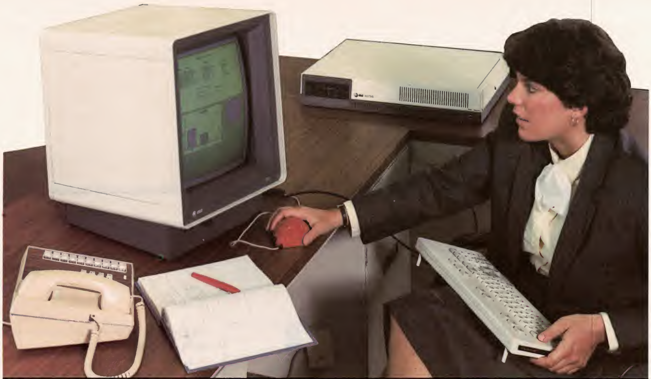
The Teletype 5620 dot-mapped graphics terminal is a common companion of the 3B2/300.
