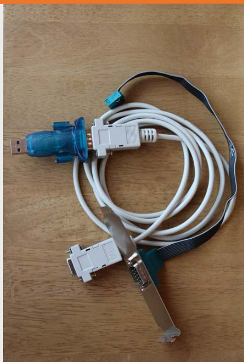
FIGURE A. A must-have toolkit to run Jailhouse bare metal: serial-to-USB converter, null modem cable (attached) and mountable COM port. (Image from Yulia Sinitsyna.)
