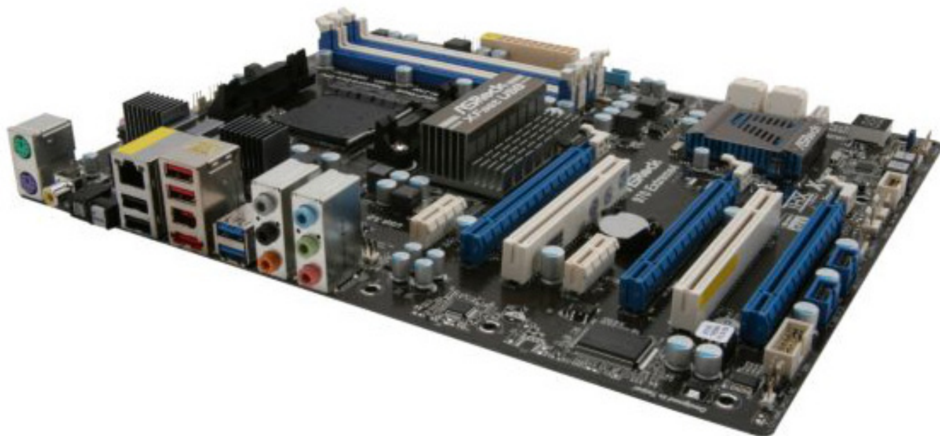
Figure 1. The PCI-E slots are far enough apart that all three are usable.
