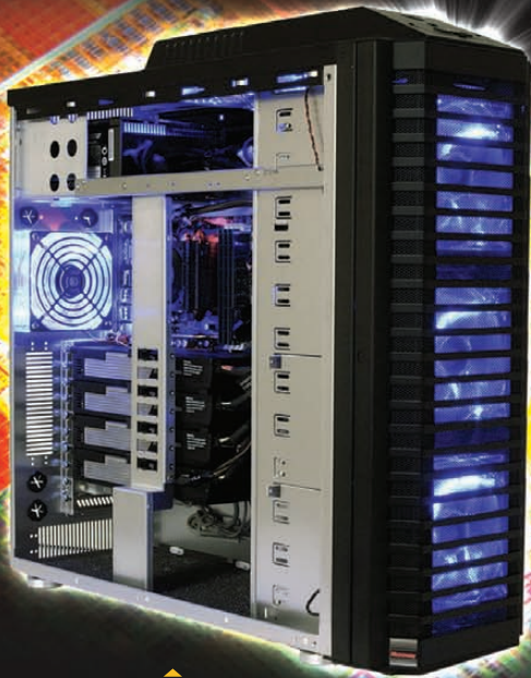
WhisperStation with 4 Tesla Fermi GPUs
