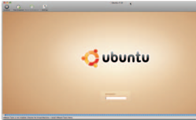
Figure 6. VMware Fusion running Ubuntu. By default, the Ubuntu virtual appliance had a ridiculously high resolution set, far bigger than the Fusion window itself. You can see that by how the login prompt isn't centered.
