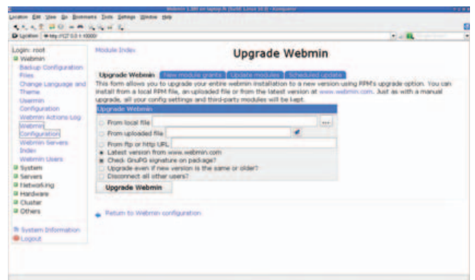
Figure 4. You can upgrade Webmin or add new modules without any other tools.
