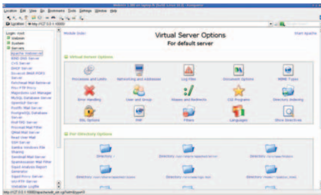
Figure 8. You can configure Apache fully with Webmin. Here, you can edit the default server attributes.
