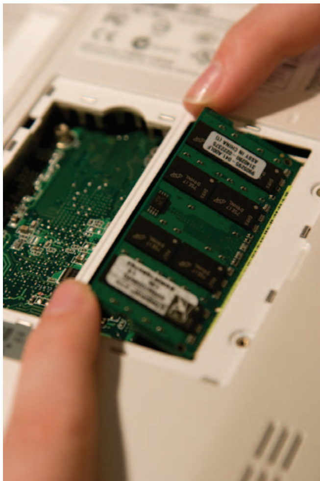
Figure 7. Installing the New Module
