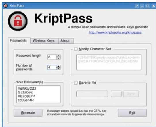
Figure 1. KriptPass is a Kommander script that provides a graphical front end to the text-based makepasswd command.
