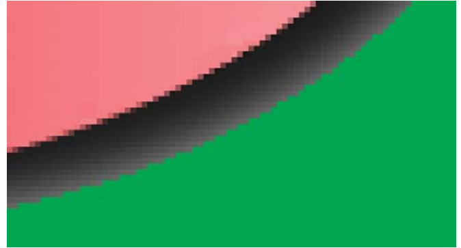
Figure 4. Button intended to have a gray background behind a soft shadow, exported with a single-bit alpha mask and overlaid on a different color background.
