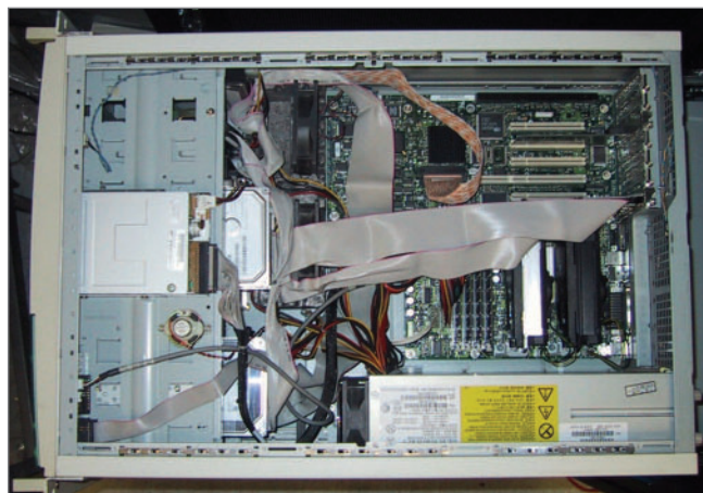
Figure 1. Storage array build from an old server (capacity of nine IDE disks, including five in a converted SCSI RAID stack). Additional IDE spots added with Promise HBA.
