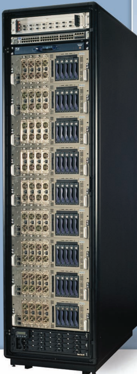
Microway® Quad Operon™ Cluster with 36 Operon 852s, redundant power and 45 hard drives in CoolRak™ cabinet.
