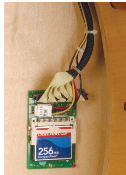
The Ultimate Linux Box boots from a CompactFlash card with an ATA adapter. Pull the card out to make an easy back-up. 256MB is plenty of space for /boot , and the rest of the storage is at the other end of a long fiber-optic cable. Going back to a noisy PC after using this machine was sure hard on the ears
