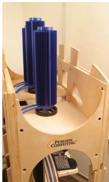
The Ultimate Linux Box has three separate cooling loops: one for the power supply and two that each handle two CPUs. We carefully monitored CPU temperatures with lm_sensors . CPU temperature rises a little before the water in the "up" tube warms up enough to start
