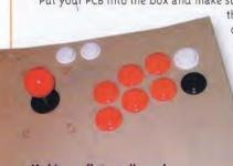
Making a flat cardboard prototype is easy and very useful for working out button positions
