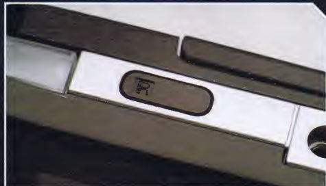
IR Window Allows for connection with any compatible IR device.
