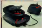
The Jaguar CD fits onto the top of the Jaguar; CDs drop into the front, carts slide into the back.
