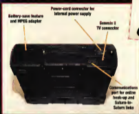
The Saturn will use a Genesis II TV connector, which means TVs without AV inputs will require a special RF adapter.
