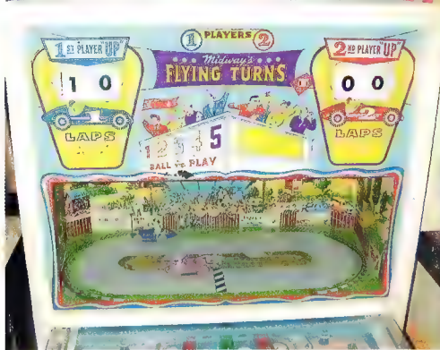
The cars actually move around the track behind the backglass in this Midway pinball machine
