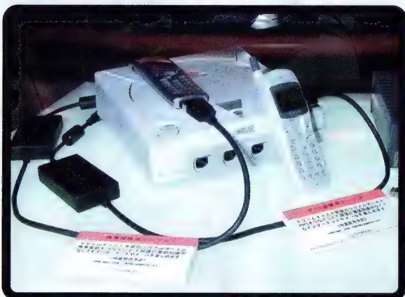
Dreamcast Cellular Phone Link – No U.S. plans have been announced, but this device allows Japanese DC owners to use their cell phone as a modem.
