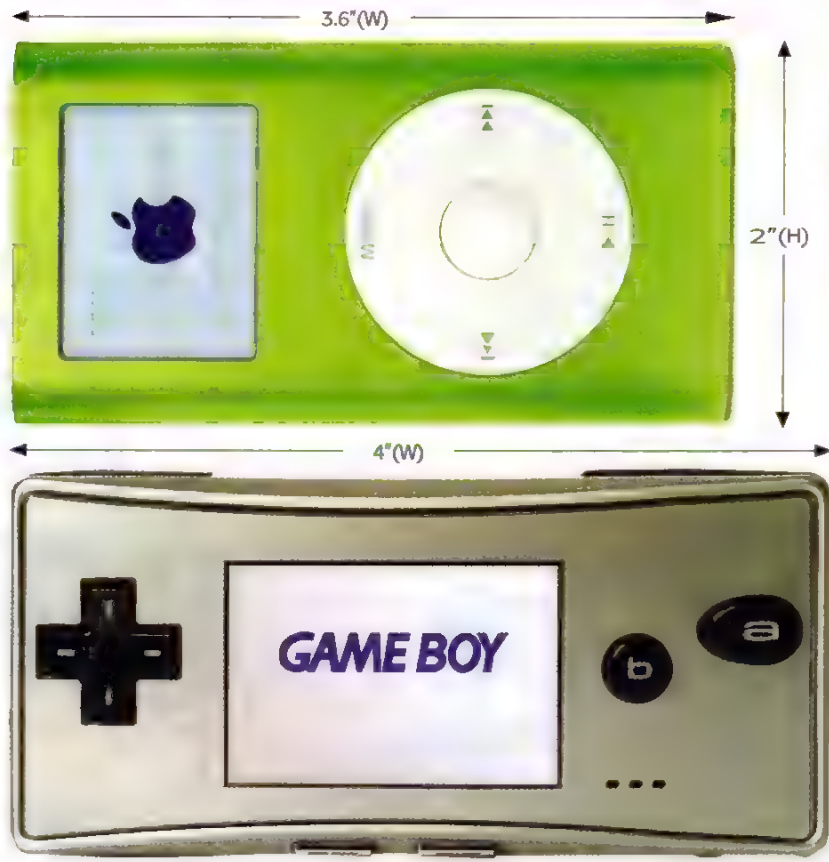
■ iPod Mini dimensions (on side) - 3.6 inches wide (the long way) and 2 inches tall. The GBA Micro dimensions - 4 inches wide, 2 inches tall
