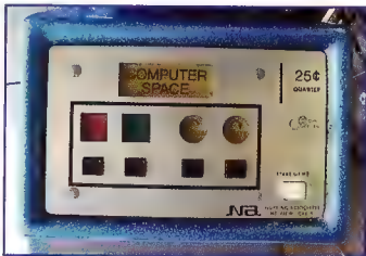
Computer Space's control scheme, which featured different buttons for thrust, rotate, and fire, proved too difficult for most arcade goers
