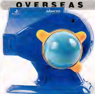
A top view of Sankyo's PS pachinko peripheral. Twisting the knob shoots balls up through the 'virtual' machine.
