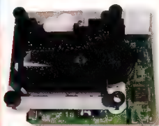
The CD drive has fewer wire connections to prevent skipping. The drive is mounted on rubber bubbles that act as springs.
