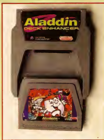
The Aladdin consists of a master module and the individual game cartridges.
