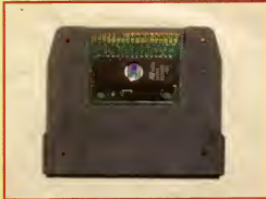
Camerica has reduced the game cartridge to its simplest form - the game chip on a board.
