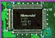
processor, it is a custom chip called the 65816. The system runs at 3.58 MHz, while not incredibly fast the Super NES can handle a huge amount of graphic information at one time. There are a total of 32,768 colors available and 256 can be displayed at any one time. The maximum res-
