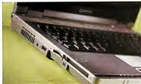
Unlike in earlier Toshiba laptops, the DVD SuperMulti Drive, TV tuner, and battery can all coexist in the Gossio—no more swapping!
