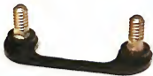
GET SCREWED This curious little gadget mounts under some new motherboards to provide support.
