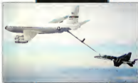
DUAL PERSONALITY Because Naval planes like this NASA F/A-18 use probe-and-drogue refueling, Air Force tankers like the KC-135 can refuel them only using an adapter on the boom.
