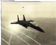
FLARE FOR COMBAT A Strike Eagle drops a flare in an attempt to distract an incoming missile.
