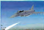
▶ EURO ATTACK The EF2000 fires a radar-guided missile at the enemy, since an infrared missile is often ineffective in head-on encounters.
