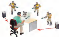
Conventional Stereo: Sounds seem to come from between speakers. Some front-to-back range.
