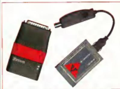
**LAPTOP CONNECTORS** The PC card NIC (right) is the least expensive means of connecting a laptop to a network. It plugs into a PC card slot and accepts an RJ-45 or a BNC connection; the Linksys PC card shown accepts both connectors. If your laptop doesn't have a PC card slot, the parallel port (null-modem) adapter (left) is the alternative, but it's much more expensive. This adapter plugs into the parallel port and accepts an RJ-45 (10-Base-T) connection.
