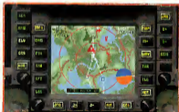
MAGIC MAP The moving map display gives you a full tactical picture of nearby air and ground activity, using data from nearby J-STARS and AWACS planes.
