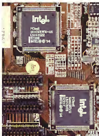
TRITON IS THEIR NAME These two chips make up half of Intel's four-chip Triton chipset. These babies control virtually all system I/O, from the hard drive to the data streaming to and from your video card via the PCI bus.
