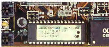
FLASH MY BIOS This rather gaudy chip is the BIOS, which tells your computer how to boot up and where to find its various parts. This is a BIOS designed for a 586 (Pentium) PCI system.
