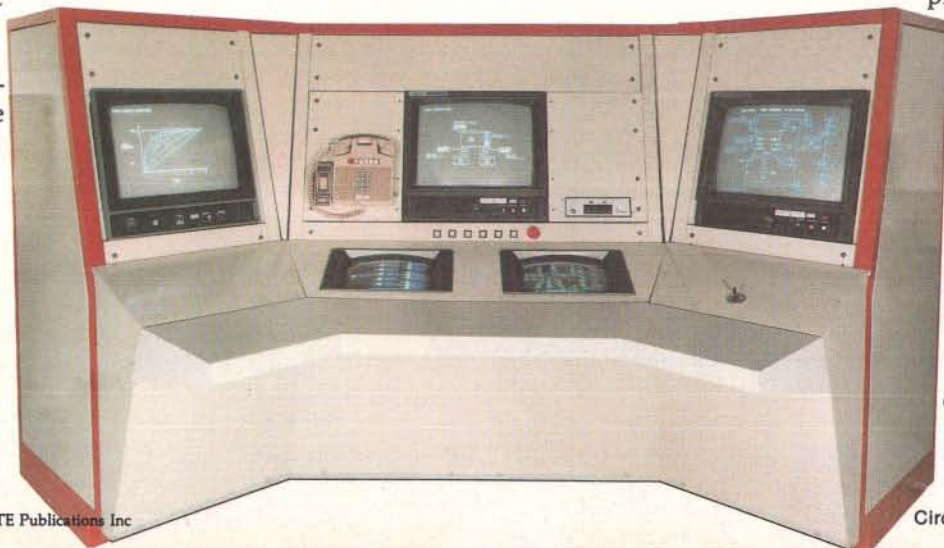
Photo 7 (below): The control panel for an experimental fusion reactor at Lawrence Livermore National Laboratory. Transparent touch panels mounted over the color video displays have eliminated most switches. To control the reactor, the operators need only to touch the screen over the desired control area shown on the screen. Photo courtesy of Glenn Spreckert.
