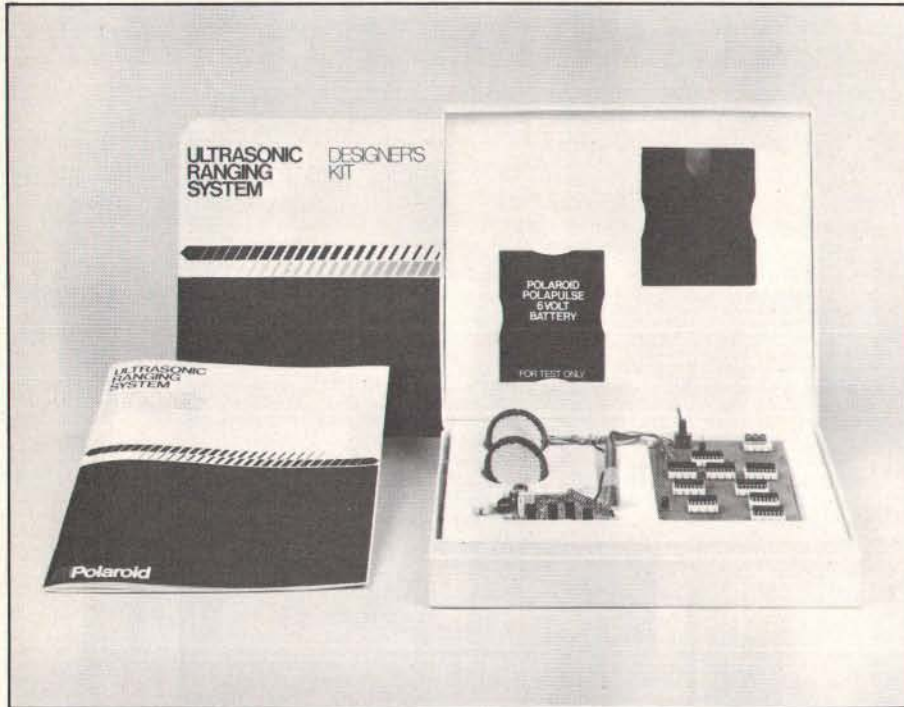
Photo 2: Polaroid Ultrasonic Ranging System Designer's Kit, which includes ultrasonic sonar transducers, electronic circuitry, and a detailed specifications booklet.
