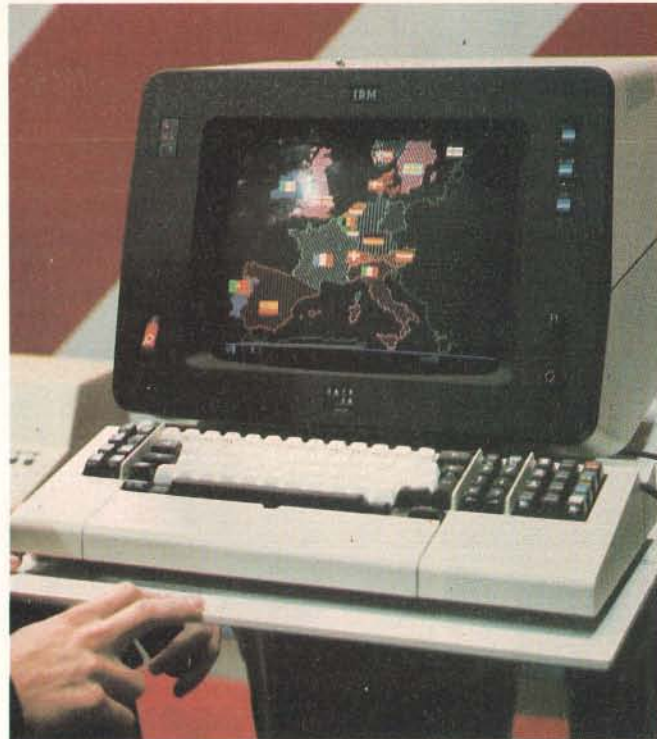
Photo 5: IBM's Model 3279 color-graphics terminal. This terminal is oriented toward business and management graphics rather than toward engineering applications.
