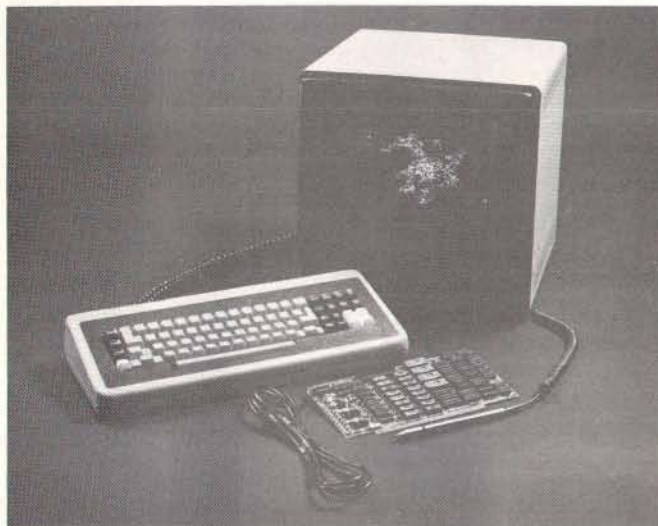
Photo 1: The MicroAngelo Graphics Subsystem. Included in the subsystem are the MicroAngelo S-100 board, the 15-inch high-resolution black-and-white monitor, and a special keyboard that has an IBM Selectric-style layout plus some special function keys on the far left and right. The light pen is optional.
