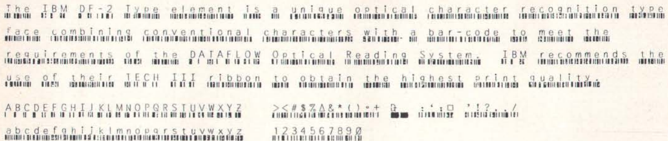
Figure 1: An example of the IBM DF-2 OCR output, using the High-Yield Correctable Film Ribbon.
