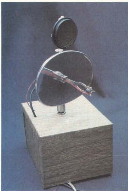
Photo 1: A computer-controlled, stepper-motor-driven infrared and ultrasonic ranging scanner. An infrared-sensitive photo Darlington transistor (GE L14F2) is mounted at the focus of a parabolic reflector, which is attached to the shaft of a stepper motor; the ultrasonic transducer is mounted above it.
