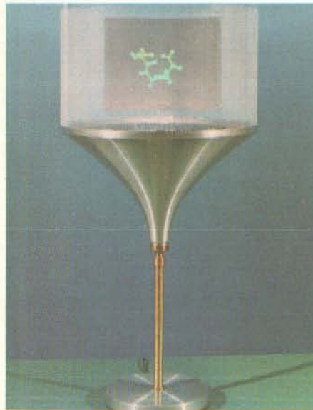
Photo 9: Integral hologram of a molecule created by photographing 1080 computer-generated images on 35mm film and then transferring them to a hologram. In the future computers will be able to generate holograms directly. Photo courtesy of Donald L Vickers, Lawrence Livermore National Laboratory.
