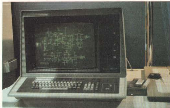
Photo 6: The Tektronix Model 4054 features a large-screen storage display tube and built-in cartridge-tape drive, with disk drives optional.
