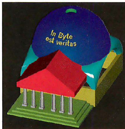
The BYTE Pantheon is a 3-D architectural model. Drawing it successfully requires surfaces, trimming tools, and a database good enough to gracefully handle a large image.
