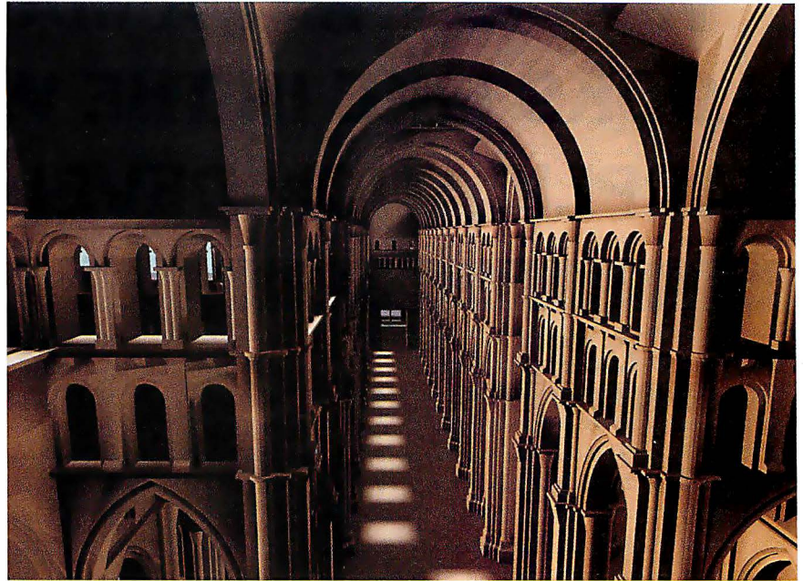
The effect of diffuse lighting is that objects that do not receive direct lighting are illuminated by the lit objects near them. The left side of the hall is lit by the light bouncing off the right side. The image was rendered using HP's Advanced Rendering Technology on an HP Apollo Series 700 TurboVRX using data generated by ASB Baudat CAD Service GmbH with IEZ Speedikon software.
