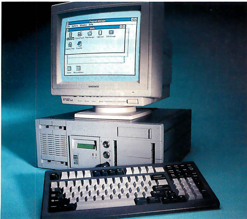
The front panel of the FTSA PC provides diagnostics messages through the LCD and access to redundant power supplies and disk drives.
