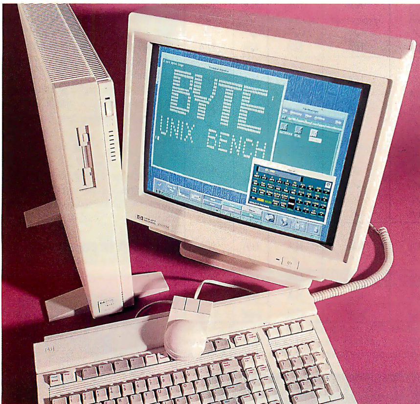
The new HP/Apollo workstations are enclosed in a small, trim case. The CPU can stand on edge (as shown) or sit flat on your desk.
