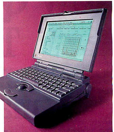
Photo 3: The PowerBook 170 delivers Mac IICI performance. Both it and the PowerBook 140 have 32-Bit QuickDraw and support for virtual memory in their 1-MB ROMs.
