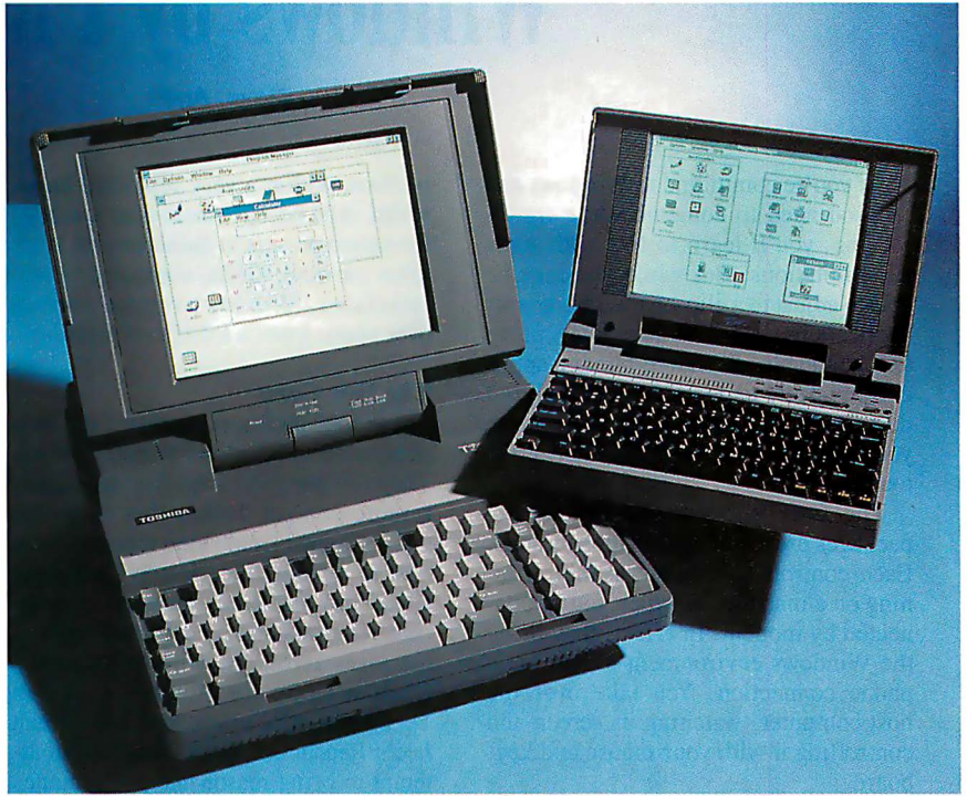
Photo 1: The Everex Tempo Carrier (right) and the Toshiba T3200SXC are both excellent machines for running Windows. The Tempo has a KeyMouse built into its keyboard for cursor control and ships with a standard mouse as well. The T3200SXC has the best color display of any portable we have seen.
