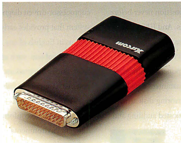
The software-switchable Pocket Token Ring Adapter II links laptops to LANs.
