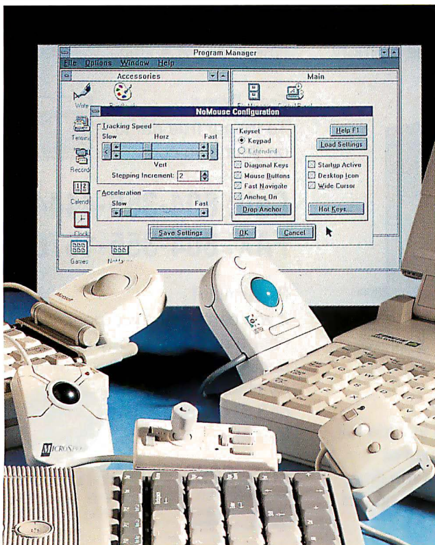
Photo 2: A litter of mice and mouse-alikes: the Abacus NoMouse for Windows (screen); clockwise from right: the Logitech TrackMan Portable, Appoint Thumbelina Portable, Suncom ICONtroller, MicroSpeed MicroTrac, and Microsoft BallPoint Mouse.
