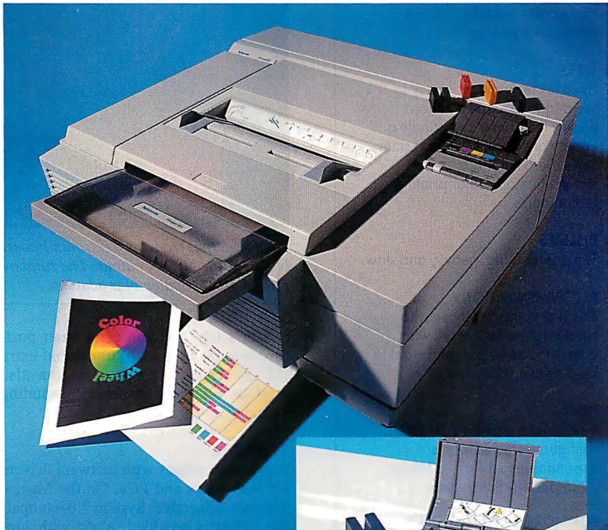
The new Phaser III color printer from Tektronix. Inset: A close-up view of the color reservoir and its keyed slots that accept the shaped solid ink blocks.
