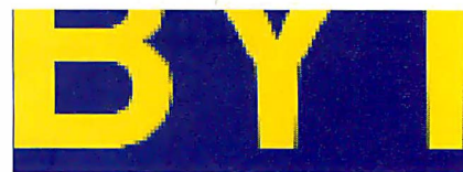
Screen 2: Although JAG does a good job of antialiasing jagged curves, such as those on the B, it also smoothes the ascenders and descenders of large sans serif type. Consequently, the base of the Y tapered at the corners and looked worse than before we ran JAG.
