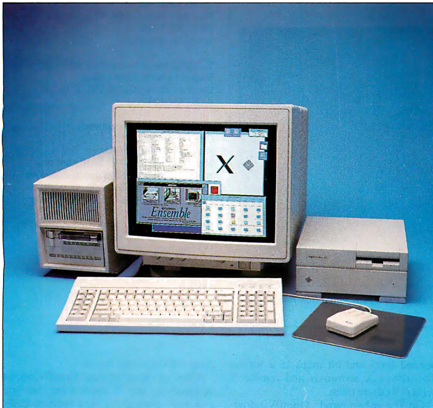
Photo 1: The Sparcstation IPC's tiny case is just large enough to hold up to 24 MB of RAM, one 3½-inch SCSI hard disk drive, one floppy disk drive, and two SBus expansion cards. The taller case is the expansion unit, housing a SCSI hard disk drive and a tape drive.
