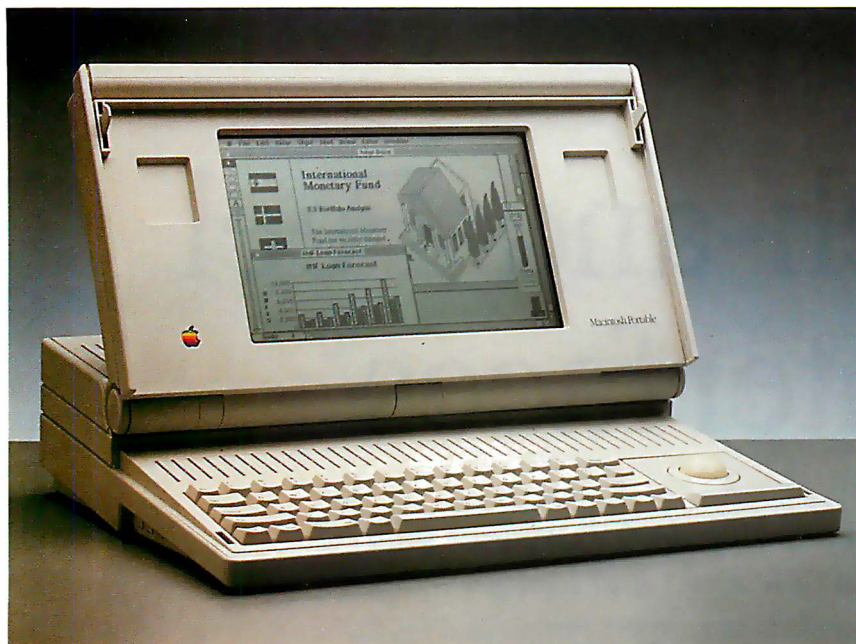
Photo 1: The Mac Portable offers a built-in trackball, which can be moved to the left of the keyboard for left-handed users or replaced with a numeric keypad. Trackballs are gaining popularity on the desktop, but they may demand too much space to be feasible for notebook computers.
