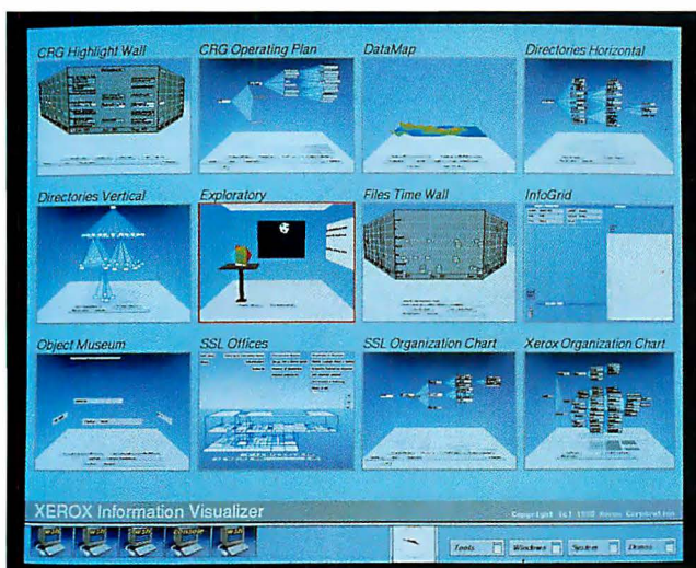
Photo 1: In the Information Visualizer system, an Overview provides a high-level look at a collection of virtual workspaces called rooms. This Overview shows eleven 3-D rooms and one 2-D room, each of which represents an active application or object that can be run and manipulated directly from the Overview.
