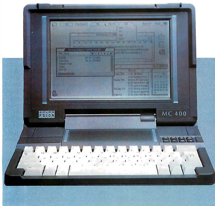
Photo 2: Psion's MC400 laptop incorporates a touchpad that lets you "point and drag" with your fingertip. The touchpad's aspect ratio is different from the screen's; it had to be squeezed in above the keyboard, so its horizontal resolution is about twice its vertical resolution.
