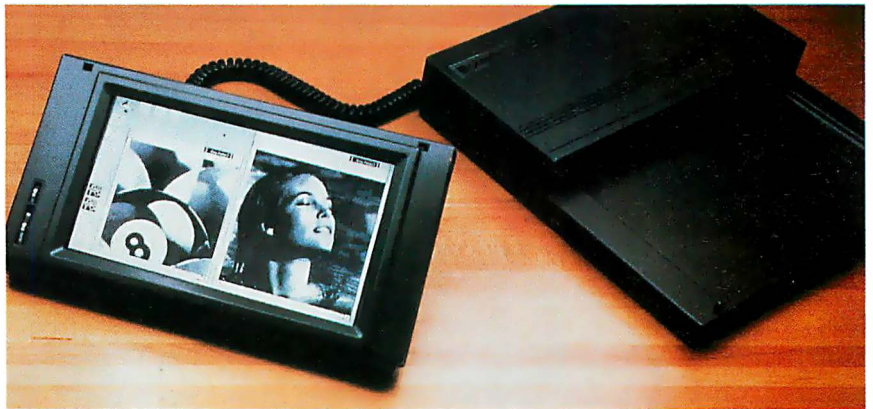
Photo 3: The Scenario DynaVision (formerly the DynaBook) is a portable information retriever with a built-in CD-ROM drive, glass touchscreen, and "point-and-shoot" query environment. The screen resolves 40,000 touchpoints, each of which has 16 levels of pressure. The machine also runs DOS programs with an optional keyboard.
