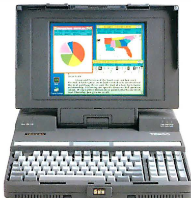
T5200C. 386 microprocessor, 200MB HDD, 2 to 14MB RAM, 2 IBM-compatible expansion slots (in addition to dedicated memory slots), VGA passive matrix color LCD display.
