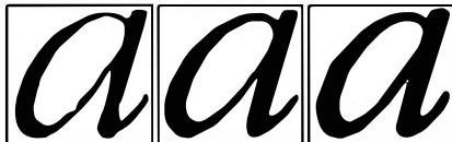
300 x 300 dpi LaserWriter II 800 x 400 dpi NewGen PS/480 600 x 600 dpi Varityper VT-600
