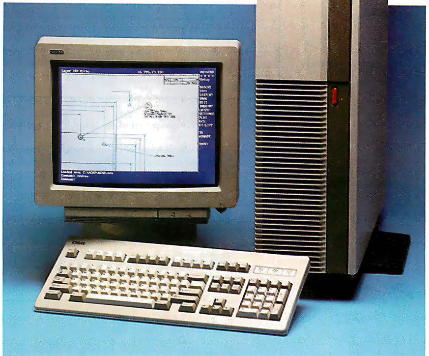
As the size of its case suggests, the NCR S486/MC33 has plenty of room for expansion. It is also one of the fastest 33-MHz 486 systems BYTE has tested.
