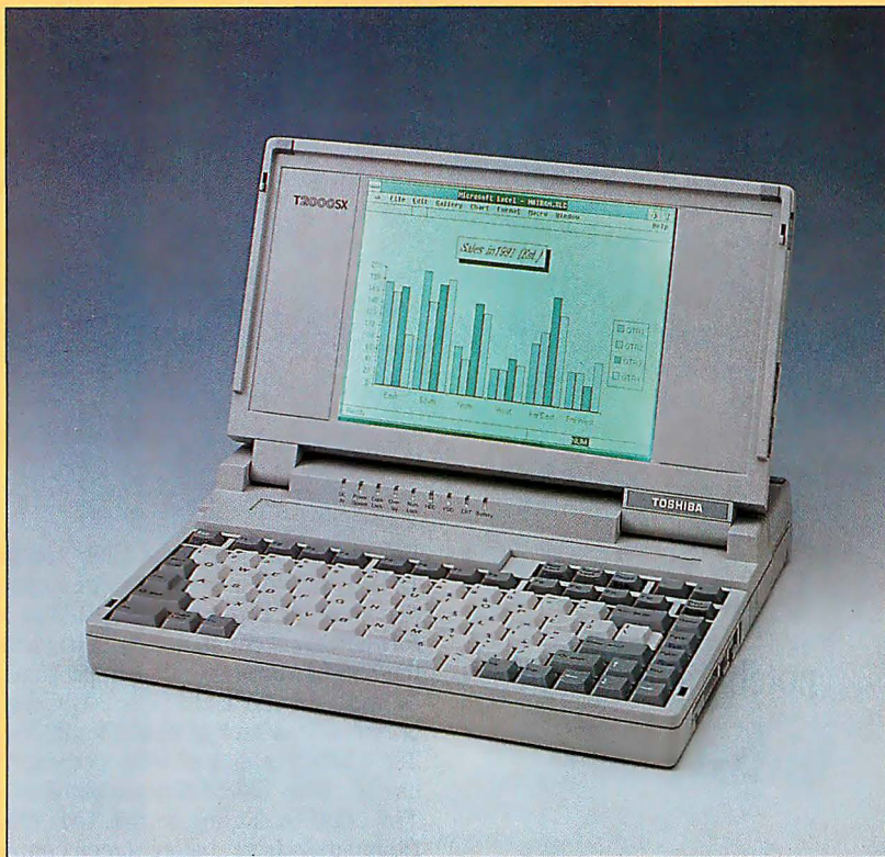
The Toshiba T2000SX is a little larger than the Texas Instruments TravelMate 3000 and uses a 16-MHz 386SX. It has the same keyboard as the Toshiba T3100SX.
