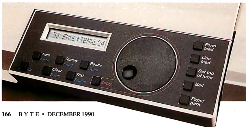
Photo 3: The Advanced Matrix Technology Accel-535 has the slickest interface of the 27 dot-matrix and page printers we reviewed this month. By spinning the dial, you can scroll through the options in the menu display. When not setting options, the dial can move the paper or set margins.
