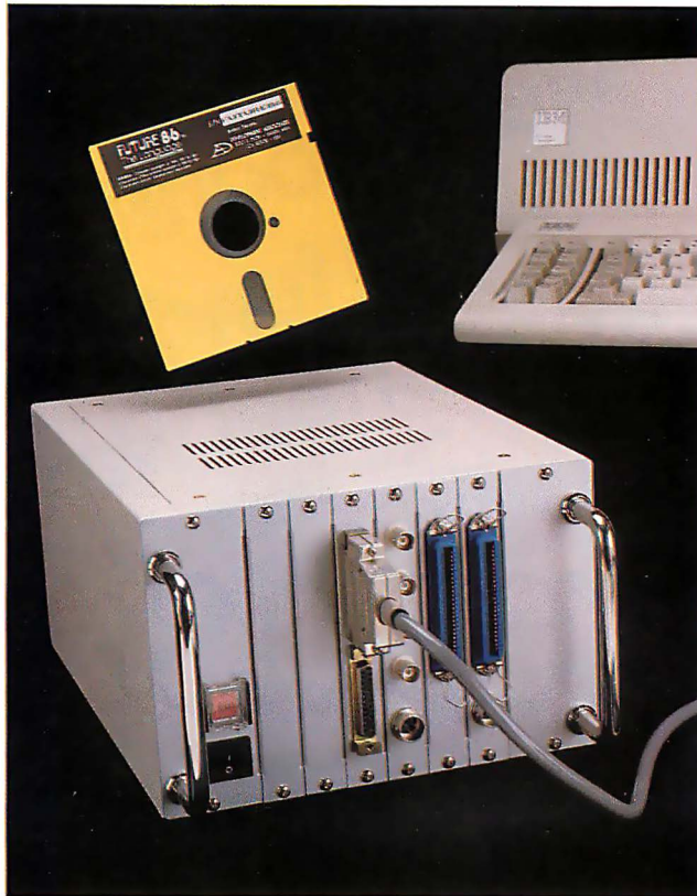
The UDM controls RS-232C and IEEE-488 I/O.
