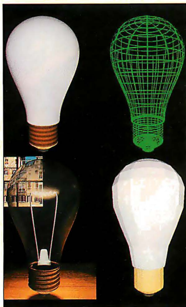
Photo A: Four light bulbs illustrate the evolution of computer graphics: (clockwise from top left) Gouraud-shaded polygons; wire-frame drawing; Phong-shaded curved primitives with texture; multiple texture and displacement mapping with transparency and shading language.
