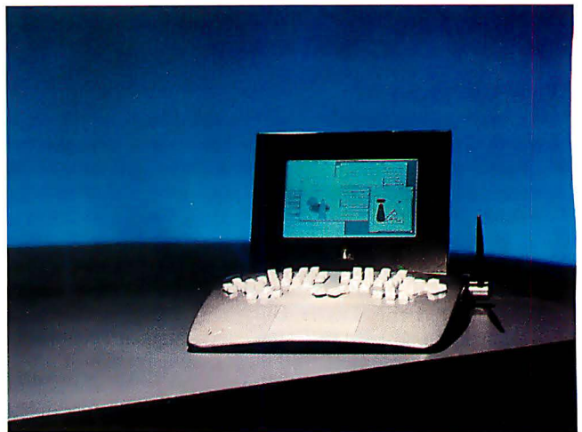
Photo 1: The BTRON standard PC includes a flat-panel display, an ergonomic keyboard, and a stylus pointing device. Everything from the CPU instruction set to the user interface was designed as a unit.
