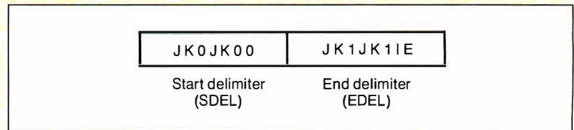
Figure D: The abort delimiter consists of a start delimiter and an end delimiter together.
