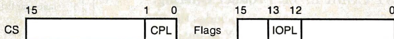
Figure 3: The CPL is located in the last two bits of the code segment's selector. The IOPL is found in the program's flags. You can modify the IOPL only when CPL=0; you can execute sensitive instructions only if CPL \leq IOPL .
