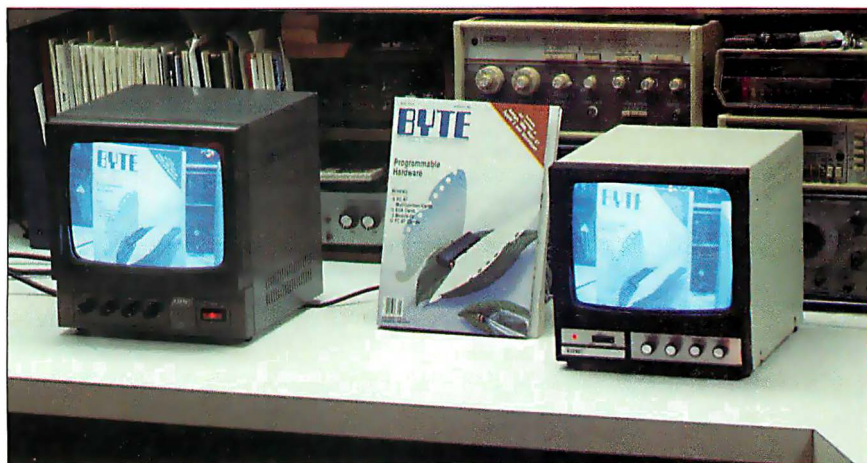
Photo 6: An in/out comparison. The camera is pointed at the magazine in the middle. The monitor on the left displays the image seen by the camera and the digitizer/transmitter. The monitor on the right shows the digitized image received by the display/receiver board.
