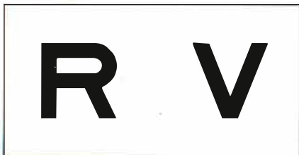
Figure 1: Two letters of the Sloan font for vision testing produced by listing 1 on a Linotype L300 at 2540 dots per inch.
