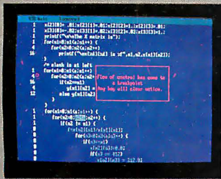
Source window with profile count showing number of times each statement has executed. Pop up message indicates break point has been hit.
