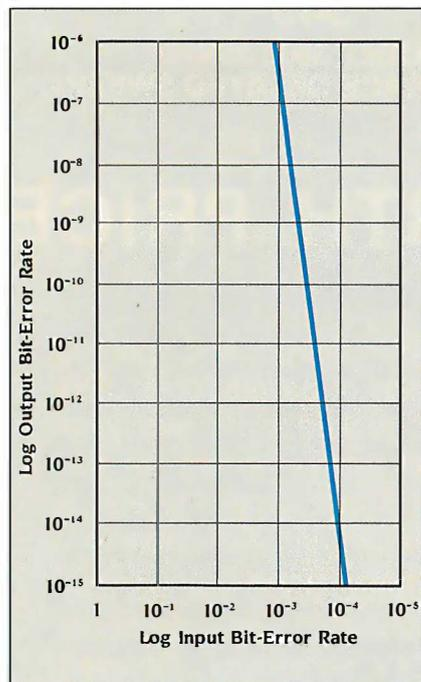
Figure 1: The relationship between the raw error rate and the corrected error rate using an RS(220,204) code. Code words consist of 220 eight-bit bytes, of which 204 bytes are information and 16 bytes are redundancy, for a code rate of 92.73 percent. The figure assumes random, independent bit errors. Performance against somewhat "bursty" errors is even better.
