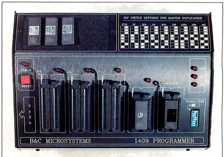
Photo 2: B&C Microsystems' enclosed model 1409C-33 EPROM Programmer.
