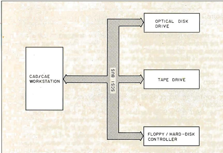
Figure 3: A single-user/multitasking SCSI system.
