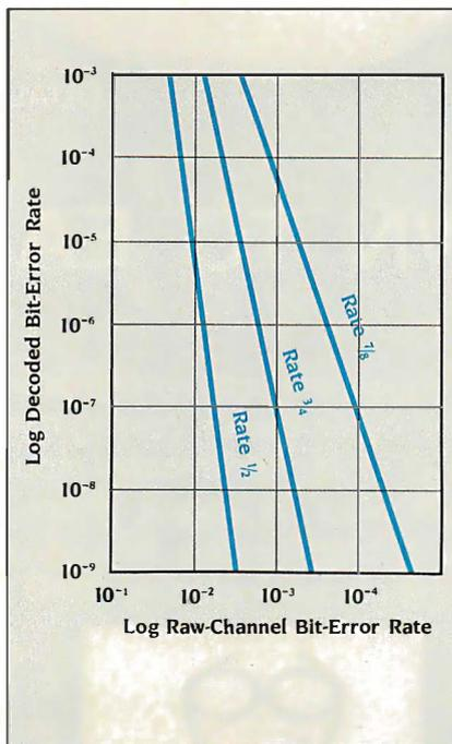
Figure 2: The performance of three RS codes against random occurrence of bit errors. All three use code words consisting of 32 five-bit bytes. The rate  $\frac{1}{2}$  code has 16 information bytes and 16 redundancy bytes per block, an RS(32,16) code. The rate  $\frac{3}{4}$  code is RS(32,24), and the rate  $\frac{7}{8}$  code is RS(32,28).
