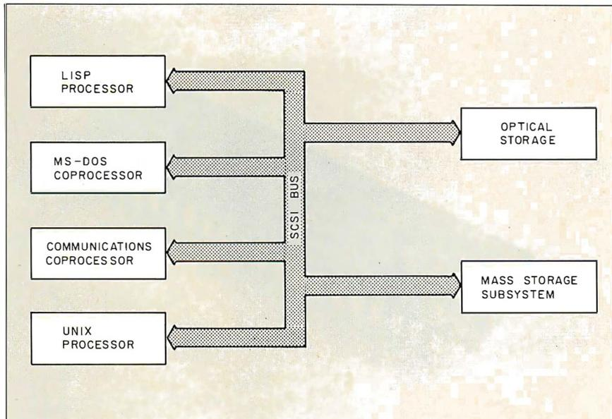
Figure 5: The SCSI bus in a multiprocessing system.
