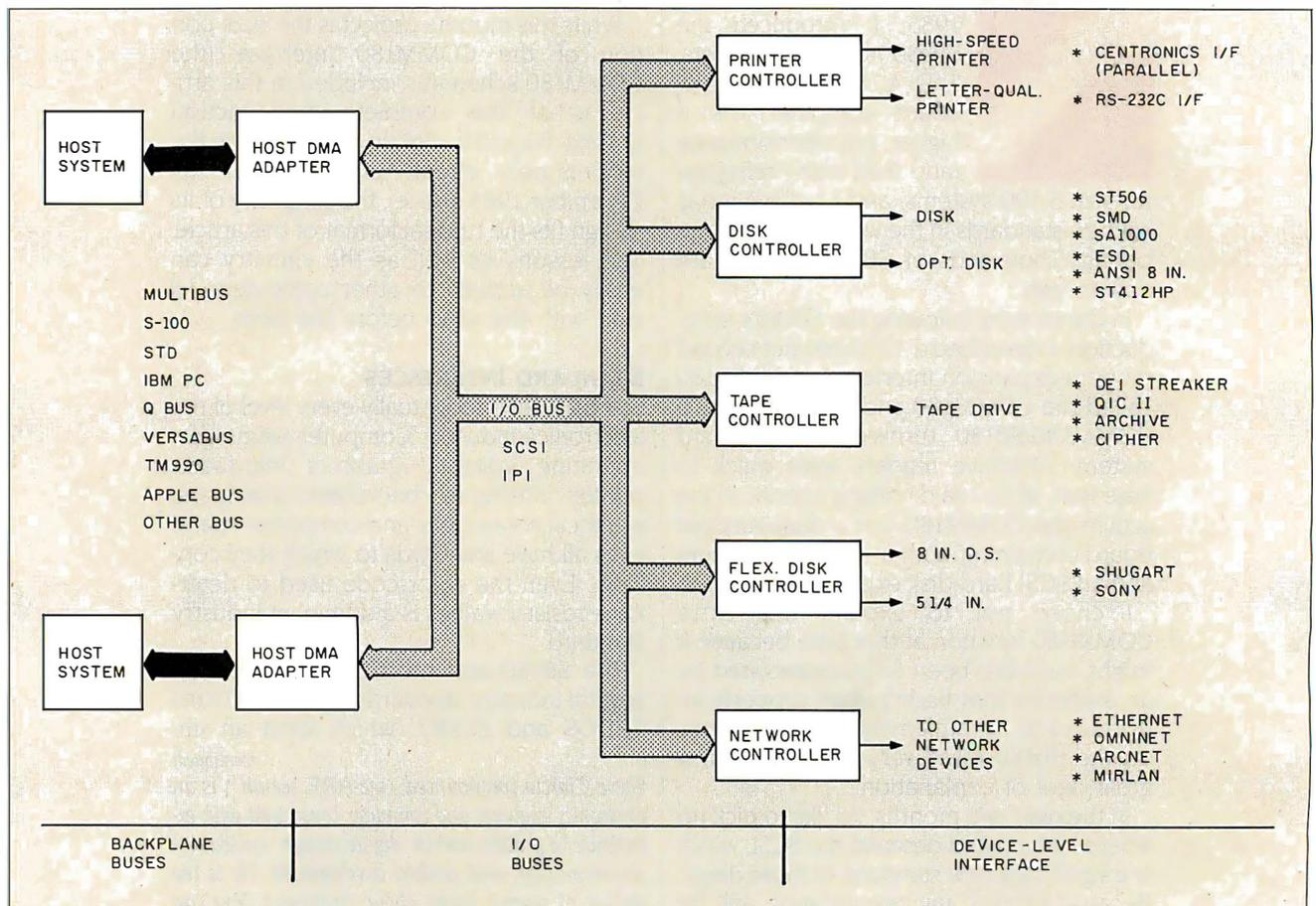
Figure 1: Computer-system interfaces.
