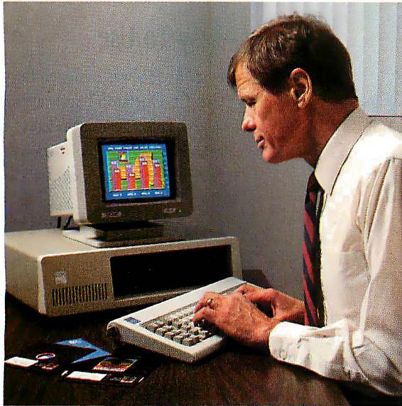
Nobody else—not even IBM—offers a 9", high-resolution RGB color display. The HX-9 and HX-9E feature a super-sharp .28mm dot pitch tube for crisp, clear text and graphics. Nonglare screens for less eye strain. The built-in tilt-and-swivel base allows you to adjust the screen to a comfortable viewing angle. Select green or amber display modes with built-in green/amber switch.
