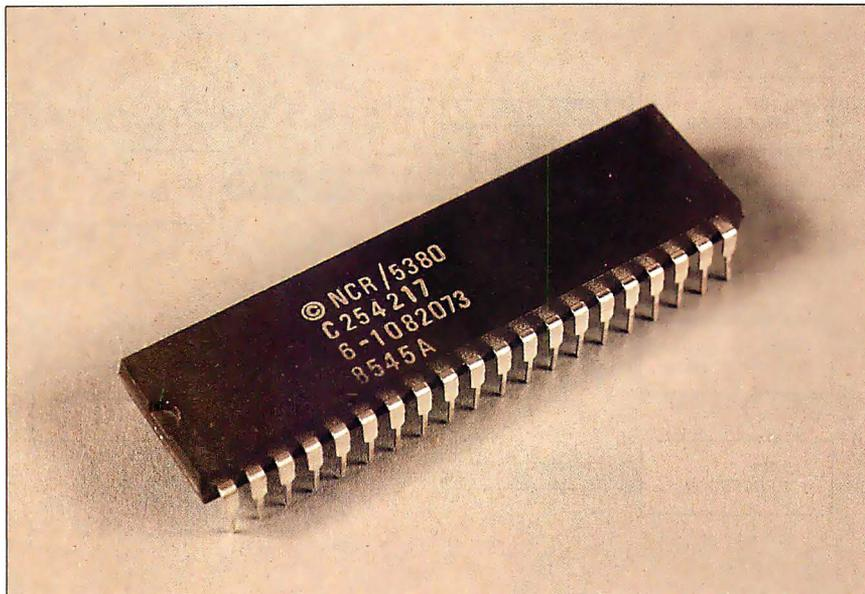
Photo 1: The NCR 5380 SCSI interface chip.
