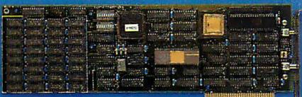
**The TurboACCEL-286 features a high-speed, 8MHz, 80286 processor, 512Kbytes of RAM (expandable to 1Mbytes), a switch for 8088 operation, and facilities for an 80287 math co-processor. It occupies one expansion slot, is completely compatible with most PCs and is software transparent. End your search for AT performance. Order the TurboACCEL-286 today! Call or write:**
