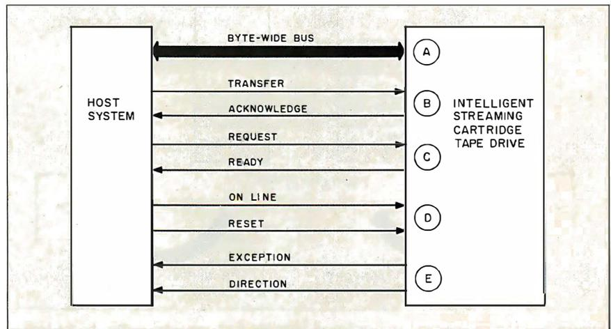
Figure 4: A summary of the typical communications between a host computer and a tape backup system, including: (a) the actual data, command, and status bytes; (b) data transfer-acknowledge handshaking; (c) command-status handshaking; (d) host-to-drive control signals; and (e) drive-to-host status signals.
