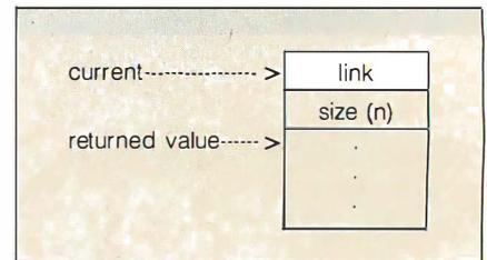
Figure 2: The returned value is a pointer equal to the current pointer value plus the size of the MemoryDescriptor record.
