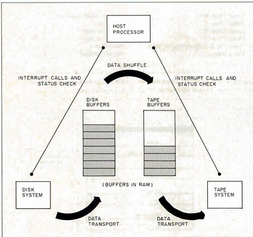
Figure 5: In the process of data exchange from the host computer system to the tape backup drive, the tape software uses the host system's RAM as a buffer to manipulate data blocks.
