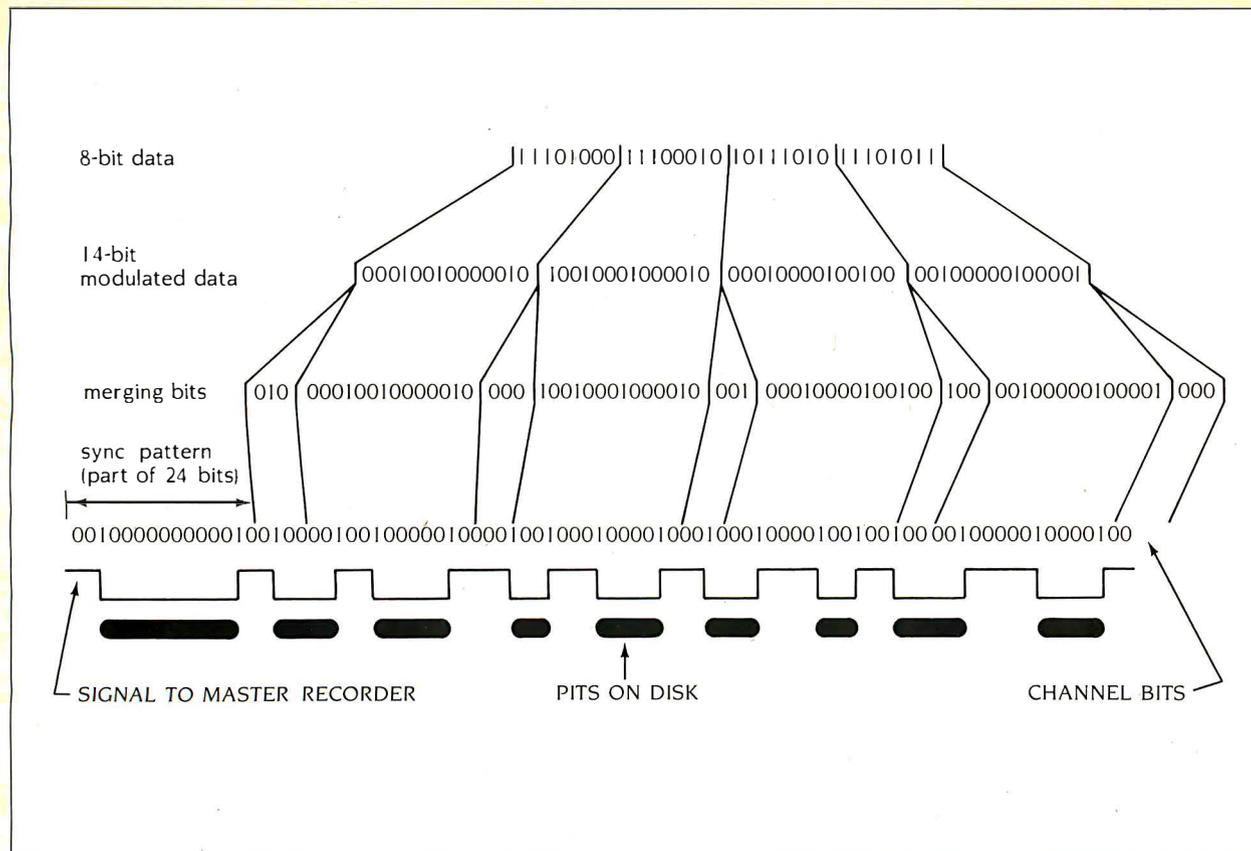
Figure B: The EFM (eight-to-fourteen modulation) process. Note the long pits burned into the disk by the laser, encoding up to ten 0s within a single pit.
