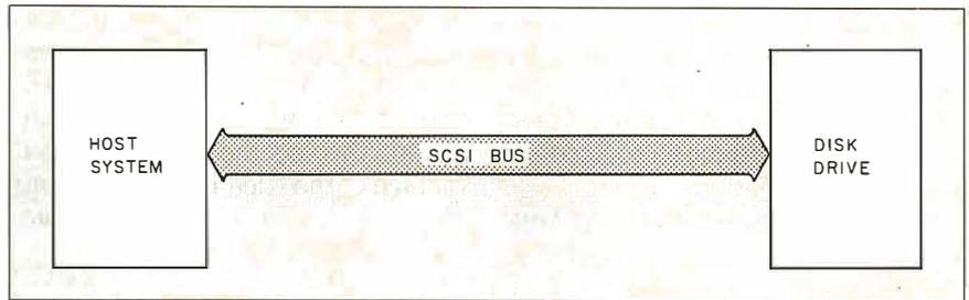
Figure 2: A simple SCSI configuration.
