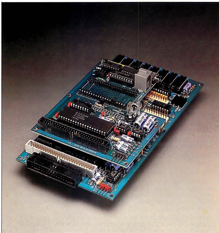
Photo 2: The COMMI80 SCSI interface board rides piggyback on the SB180 single-board computer. The NCR 5380 is the large chip toward the front. Note the empty socket for the MOSART modem chip (see the November 1985 Circuit Cellar for a description of the MOSART).
