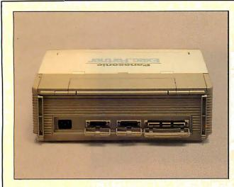
The back of the Exec. Partner showing, from left to right: power plug receptacle, parallel port, serial port, and expansion connector.
