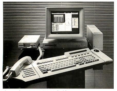
Photo I: The new Apricot XEN 80286-based business microcomputer. It is shown with a 360K-byte 5¼-inch floppy-disk unit and an expansion box, which can house up to two IBM expansion cards; these units provide some compatibility with the IBM PC and the PC AT. The optional combination trackball/mouse and telephone are also shown. The XEN is seen running Microsoft Windows, which is its standard operating environment.
