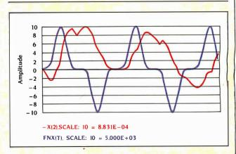
**Figure C:** A graph of displacement (X(2)) and driving force (FNX(T)) versus time for a system with Coulomb damping and nonlinear spring force.
