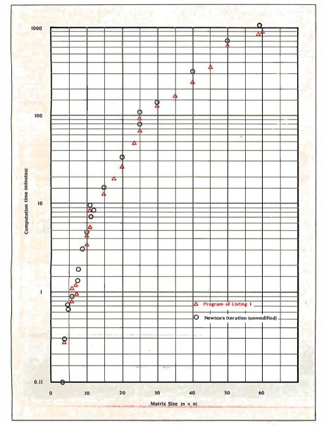
Figure 3: A plot of log (computation time) versus matrix size.
