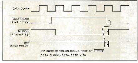
Figure 2: RAM load timing.
