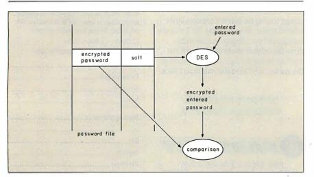
**Figure** 4: UNIX password verification. The entered password is encrypted by a variant of the DES algorithm using the salt string readout of the /etc/passwod file entry for that user. The resulting encrypted password is compared to the encrypted password in the file. If they are the same, the password is accepted. Note that the password in the file is never "decrypted."
