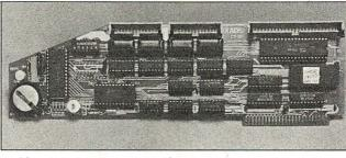
Xcalibur's XAD5 data-acquisition board.
