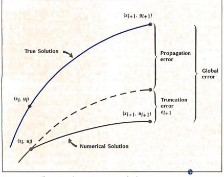
Figure I: An illustration of errors in a numerical solution.
