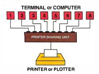
Our 4 or 8 port Printer Sharing Units work automatically. No cable switching or knobs to turn. Software changes are usually unnecessary since they use standard Ready/Busy or XON/XOFF handshaking.
