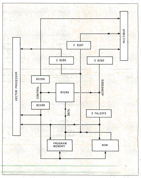
Figure 3: The configuration of the 80286, its program memory, and the Multibus interface.
