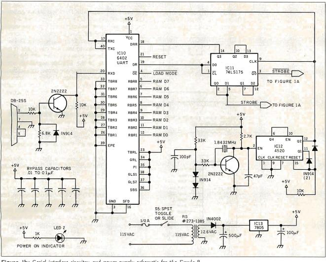
Figure 1b: Serial interface circuitry and power supply schematic for the Emulo-8.
