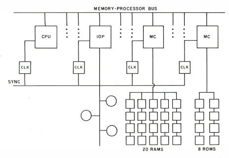
Figure 1: A block diagram of the Hewlett-Packard Focus microprocessor.
