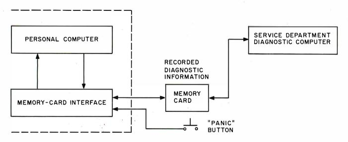
Figure 6: A block diagram of an active memory card used as an on-board diagnostics device within a microcomputer.
