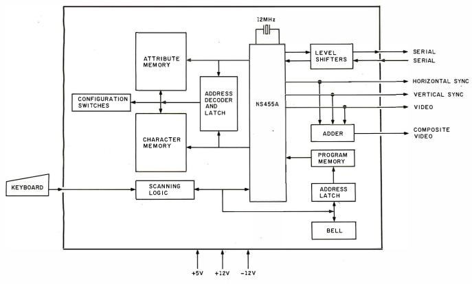
Figure 2: A block diagram of the Term-Mite ST terminal circuit board.
