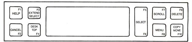
Figure 1: The Gavilan computer's control area.
