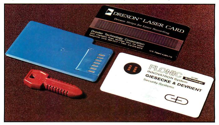
**Photo 1:** Four memory cards incorporated into different carrier packages. The bottom three cards are active devices, containing embedded microcomputers. Note the metal contact points on their surfaces (or: the "key," the contacts are between the ridges). The top card is a passive device that uses an optical stripe for laser recording and playback.
