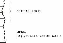
**Figure 4:** The physical layout of an optical-stripe memory card. The material on its surface is similar to that used on laser videodisks. A laser is used to read and write the transaction information.
