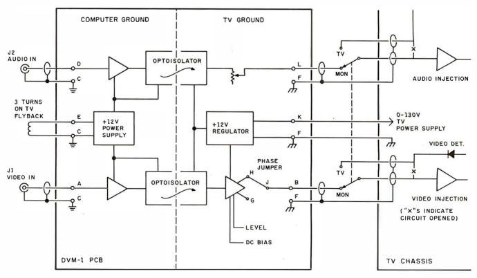
Figure 1: The DVM-1 block diagram, showing interface wiring.
