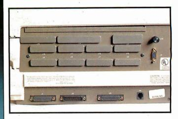
**Photo 6:** Part of the back panel of the Z-100. Along the bottom are two serial connectors (both male and female), a parallel printer port, and a light-pen connector. On the upper right is a brightness control for the internal display, just above a connector for an RGB monitor. Note the wealth of cut-outs for optional connectors.
