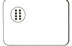
**Figure 1:** A typical arrangement of the contact points of an active memory card. Relatively few (six to eight) contacts are needed because the data is transmitted serially. See the Flonic security card in photo 1.
