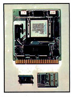
**Photo 2:** The assembled BPK 72 with the 7110 Megabit Bubble Memory installed. The seed module (bottom left) is used to restore missing seed bubbles. The dummy module (bottom right), an electrical equivalent of the bubblememory chip, is used for tests.
