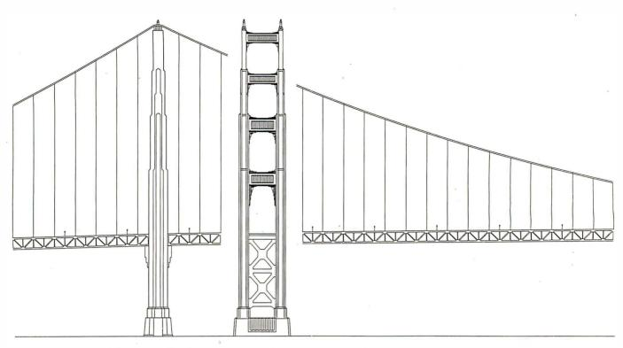
**Figure 3**: An image of the Golden Gate Bridge drawn with high-resolution, floating-point, vector-based AutoCAD software and plotted on a high-resolution Houston Instrument DMP-42 plotter.
