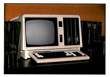
Photo 1: The TRS-80 Model 16B standard system.
