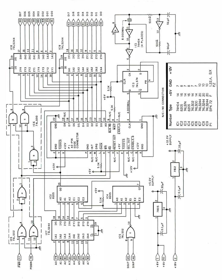
**Figure 2:** A schematic of an S-100 interface and clock circuit for the BPK 72. The kit is used as though it were a single component. Only the edge connector is shown in this figure. The schematic placement of the edge-connector pins matches that of the actual physical component. The completed project functions as either a disk emulator or a cache memory system.
