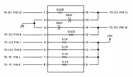
**Figure 4:** This top view of the DIP header wiring diagram includes all the resistors and capacitors (except power-supply bypass capacitors) shown in the figure 2 schematic. All resistors are 1/4 watt.
