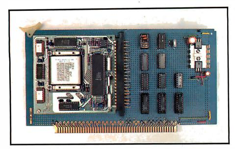
**Photo 3:** The completed S-100 bubble-memory board's component side with the BPK 72 installed (see figure 4 for the parts layout).
