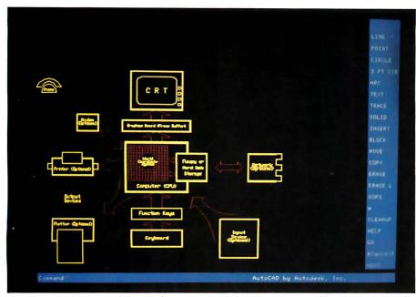
**Photo 3:** The hardware elements of a CAD system drawn using vector-based AutoCAD software and displayed by a 640 by 400 Vectrix Graphics processor and high-resolution Vectrix color monitor. Note that much of the configuration is optional.
