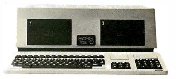
**Photo 1:** The Basis ("Bah-zis") 108 is a microcomputer, configured like an Apple II, with Z80 and 6502 microprocessors and 128K bytes of RAM. The 108 comes with two Basis disk drives. The earlier model (shown here) has Micro-Sci drives. The keyboard provides all the features required of a business system.
