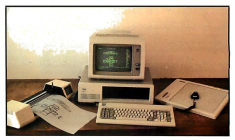
**Photo 4:** One example of a CAD system, an IBM PC with a Houston Instrument Hipad 11 by 11 digitizer and DMP-40 plotter.
