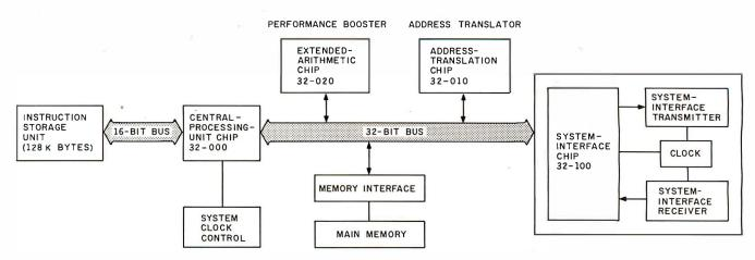
Figure 3: A configuration of the NCR/32 System.
