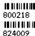
Figure 1: Bar codes generated by a Centronics 737 dot-matrix printer and a TRS-80 computer, using the program in listing 1. The program also prints the equivalent Arabic numerals under the code.
