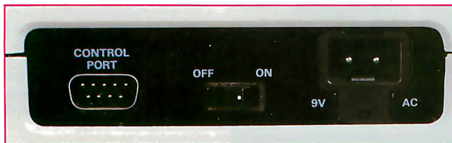
Photo 2: Connections to the VIC 20 microcomputer. Photo 2a shows the rear panel of the VIC; from left to right are a slot for program cartridges and connections to a television or video monitor, a floppy disk, a Commodore cassette recorder, and a printer or other peripherals. Photo 2b shows a game device port, an ON/OFF rocker switch, and a connector for an external power supply.
