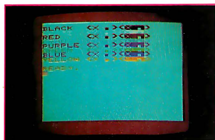
Photo 6: Variations in character, background, and border colors on the VIC 20. Photos 6a and 6b differ only in the value stored in location 32,879, which determines the background color (from sixteen choices) and the border color (from eight choices).
