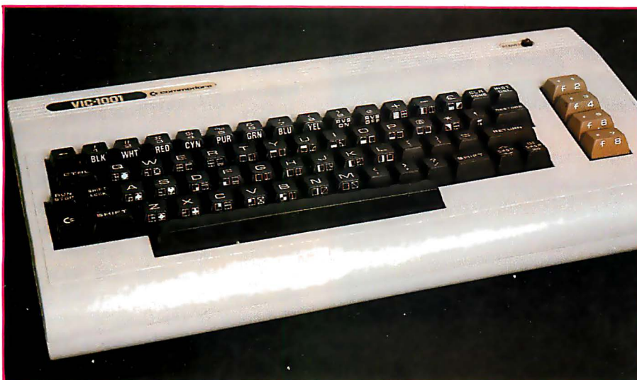
Photo 1: The Commodore VIC 20 microcomputer. This unit, a final prototype based on the Japanese version of the VIC microcomputer, differs from the American model only in the model number.
