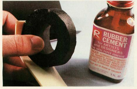
**Photo 5:** Adding pliable material to produce a tight fit around the phone handset. I found a plastic placemat at a discount store with a  $\frac{1}{16}$ -inch foam backing that was perfect. Cut a strip  $1\frac{1}{12}$  by 8 inches and glue this around the outside of the wedge as shown. Trim to the exact circumference and cover with a strip of fabric adhesive tape. The latter helps hold everything together.
