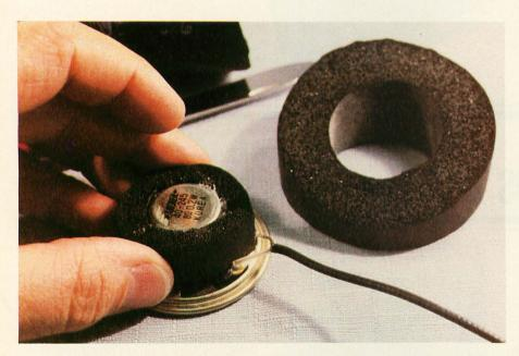
**Photo 3:** First of a series of photos (3 thru 9) showing how you can easily contruct an acoustic-coupler pickup. My design for the pickup uses such "exotic" materials as a hotwater pipe foam insulation, a pair of 2-inch, 8-ohm dynamic speakers, a foam-backed dinner placemat, rubber cement, and adhesive tape.
