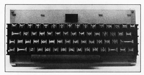
**Photo 3:** The sixty-three-key Jameco keyboard mounted on its printed-circuit board and installed on support blocks.
